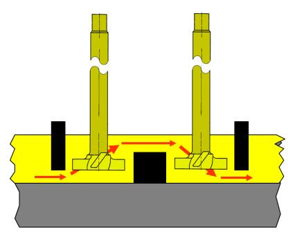
A combination of skimmers and a barrier wall create a vertical flow component in the mixing area
